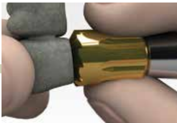
Use the reamer to eliminate the "Lip" created by the "snap-on" mechanism.
