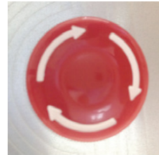
Appearance of Emergency Switch
