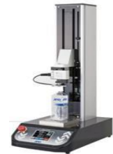
Universal testing machine Measures toothbrush's tensile strength
